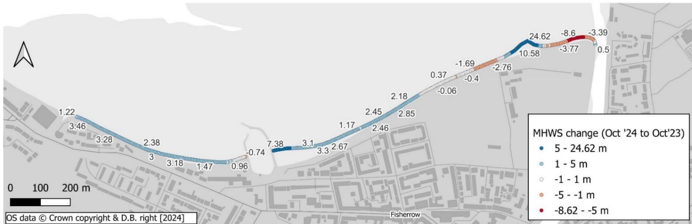
Figure 3 Changes to MHWs between October 2023 and October 2024. Points symbolized to reflect coastal change over the preceding year, annotation shown at ca 50m intervals, in metres of change.
